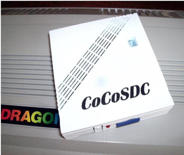
The CoCo SDC plugs into the cartridge port of the computer, replacing the Disk controller and disk drives.
